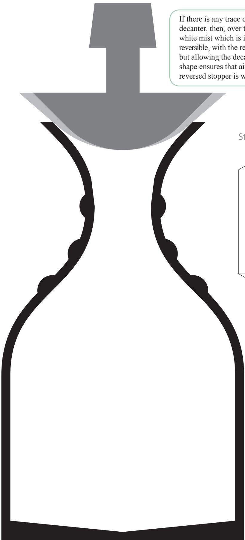
If there is any trace of water in a sealed and otherwise empty decanter, then, over time, the inside of the glass will acquire a white mist which is impossible to remove. So the stopper must be reversible, with the reversed stopper preventing dust from entering but allowing the decanter to 'breathe'. The stopper's hexagonal shape ensures that air can get around the reversed stopper, and the reversed stopper is wide enough to cover the lip completely.
