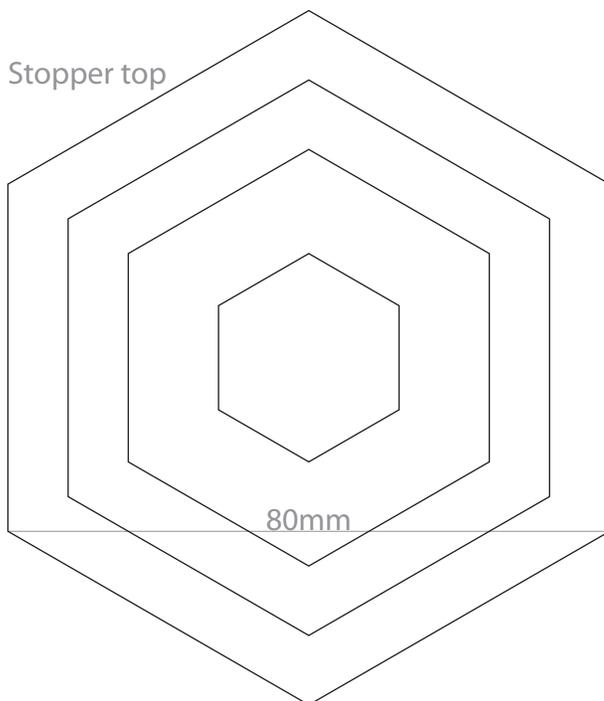
The stopper must not roll. A stopper placed on the table must rest where it is placed: it cannot be a ball. The hexagonal top of the stopper further prevents on-table movement.
